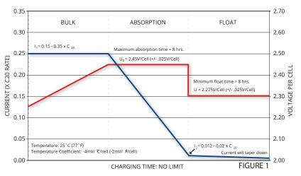
The initial charge current is recommended to be set at 0.20 x C in order to fully charge the batteries within a reasonable amount of time. It can be set lower; however, please be aware that charge time will increase so make sure the batteries have enough time to fully charge before being put back into service. Fullriver batteries have a low internal resistance allowing them to be charged at a higher current, therefore faster, than conventional flooded/wet batteries.
